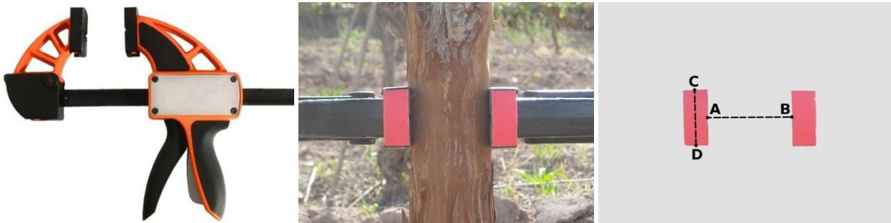
Figure 1. From left to right: (a) Quick clamp; (b) Original image with the quick clamp; (c) Results obtained by the GMM segmentation algorithm for the original image and calculating the distance in pixels between the spade pads (points A-B) and height in pixels of a spade pad (C-D points).
